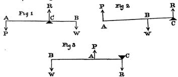
69. To find the condition of equilibrium in a simple lever and the pressure on the fulcrum, when P and W are parallel. (See figs. Art. 68).
